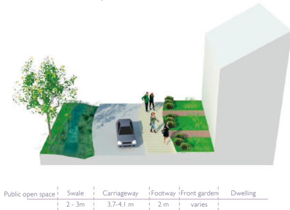
Fig 24 : Minor Residential Street Example 2
